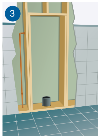
3 Route the drain and supply; prepare the wall studs.
